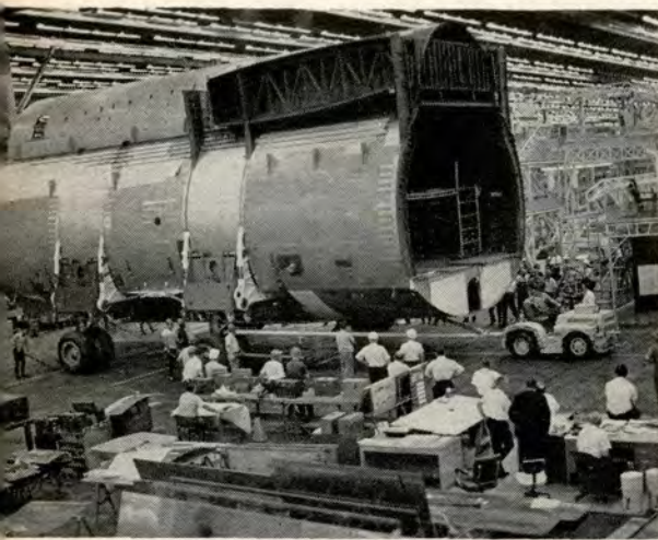
A glimpse of the future. Mid-fuselage section of huge C-5A, next generation of airlift aircraft to become operational in 1969.
